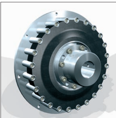
CENTAMAX-B for slight misalignment T = 0,25 - 20 kNm
