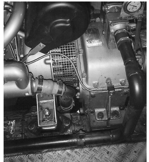
CENTAMAX-B for main propulsion between Diesel engine on soft mounts and marine gear on rigid mounts.
